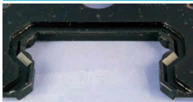
Lip has not been fractured
